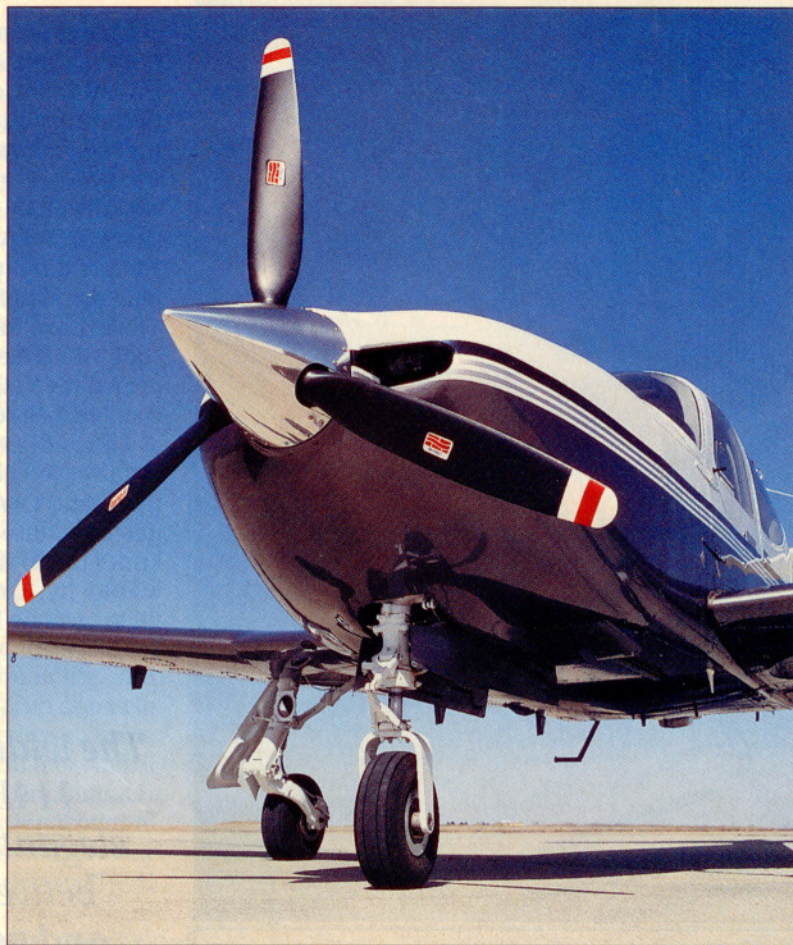
The 114B's elegant nose contrasts the tall and rugged trailing link landing gear.
